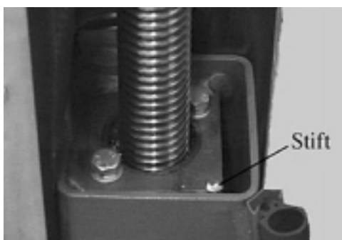
Pic.10: the carrying-nut pin (stift)
