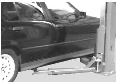
pic1: Position the pads under the described points of the vehicle.
